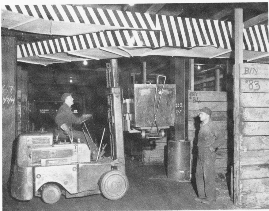
This overhead duct was almost invisible. As a result, it was hit frequently by lift-trucks. Henri Fontaine, operating the truck, and Bill Secula, of the Casting Shop Scrap Room, say that the Paint Shop did a good job. The duct now "screams" at them long before they get near it. Color is just one more thing that is being harnessed for our benefit. It can stimulate or soothe, and it may irritate or scream, if not judiciously applied. This is a good example of color as an aid to safety.
